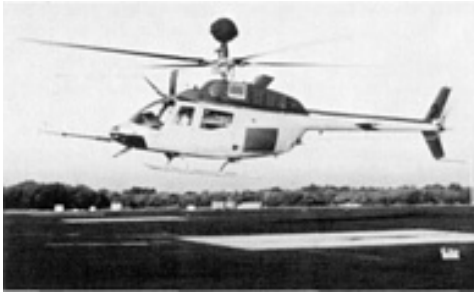
Fig. 4 Mast-mounted sight system (positioned above rotor) using a beryllium optical bench
