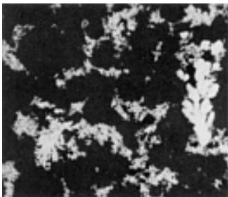
Fig. 13 Electrolytic copper powder showing dendritic structure. 85 \times . Source: Ref 9
