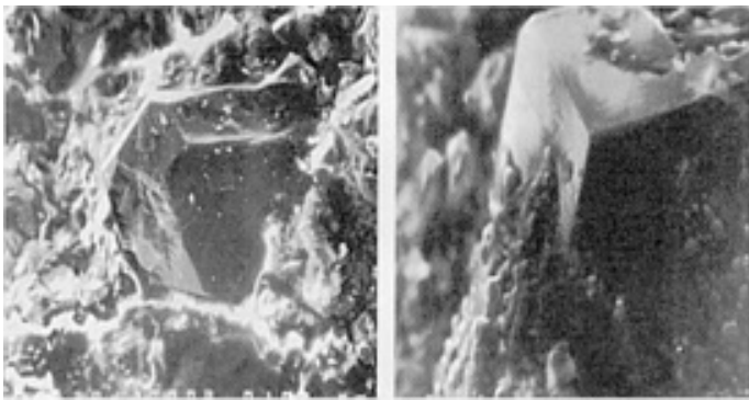
Fig. 16 Characteristic microstructure of the diamond-containing region in a Ni-Al diamond composite produced by self-propagating high-temperature synthesis. Reprinted with permission. Source: Ref 137
