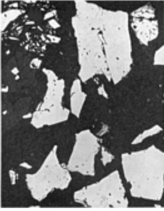
Fig. 1 Cross section of +40 mesh ground magnetite. 30×
