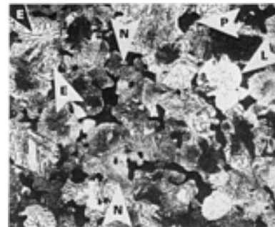
Fig. 100 Same as Fig. 99, but with 0.8% C. Arrows N show nickel-rich areas containing platelets of martensite or bainite. Arrow L indicates a light-etching eutectoid region, and arrow P a pore. Arrows E outline a colony of eutectoid containing thin carbide platelets. 2% nital. 330×
