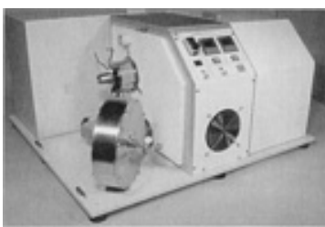
Fig. 6 Uni-Ball-Mill with the provision of a spatially adjustable high strength magnet. Courtesy of Australian Scientific Instruments, Fyshwick, Australia
