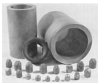
Fig. 21 Tungsten-carbide/cobalt parts produced by HIP. Source: Ref 22
