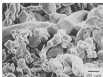
Fig. 1 Sponge fines made by the Hunter process
