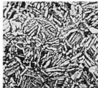
Fig. 125 Ti-6Al-4V, cold isostatically pressed, vacuum sintered, then hot isostatically pressed to 99.6% density. Structure shows all transformed \beta . 85 mL H 2 O, 5 mL HNO 3 , and 10 mL HF. 180×. (Ref 13)
