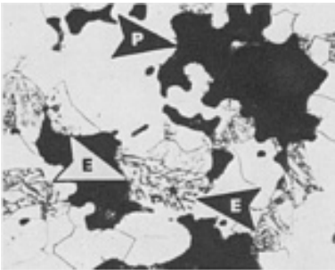
Fig. 73 Prealloyed low-alloy steel (Fe-0.42Ni-0.62Mo-0.2C, 6.7 g/cm 3 ), pressed at 410 to 480 MPa (30 to 35 tsi) and sintered 30 min at 1120 °C (2050 °F) in dissociated ammonia. Arrows E surround eutectoid region (background is white ferrite). Arrow P shows a pore. See also Fig. 74 and 75 for effects of increasing carbon content. 2% nital. 545x
