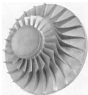
Fig. 10 Gas turbine engine compressor rotor made from hot isostatically pressed plasma rotating electrode processed Ti-6Al-4V powder
