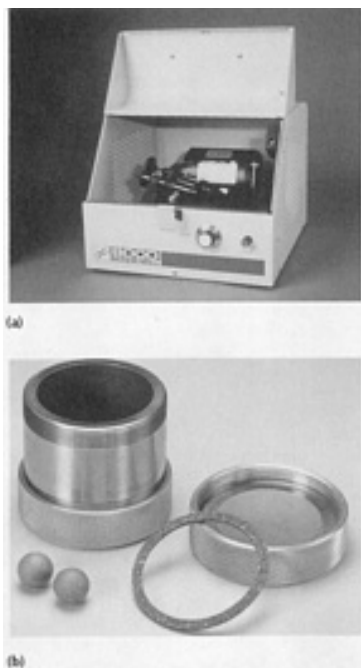
Fig. 2 (a) SPEX 8000 mixer/mill in the assembled condition. (b) Tungsten carbide vial set consisting of the vial, lid, gasket, and balls. Courtesy of SPEX CertiPrep, Metuchen, NJ
