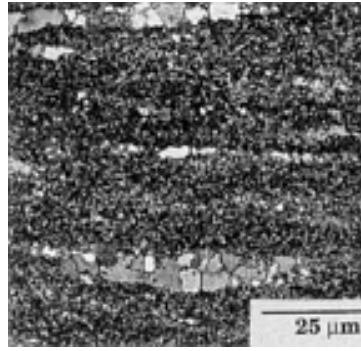
Fig. 6 Abnormal grain growth in 15 nm iron close-die sintered at 810 K (10 MPa, 1 h) followed by pressureless sintering at 1080 K for 1 h. Source: Ref 10
