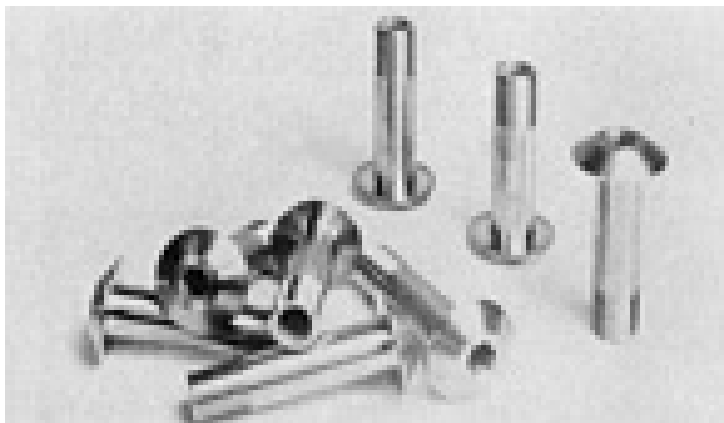
Fig. 7 Hollow bolts. Courtesy of Imperial Clevite Technology Center
