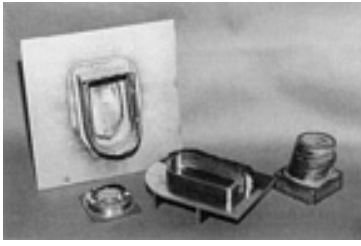
Fig. 12 Thick-walled Ti-6Al-4V laser-based direct fabrication. Source: Ref 41
