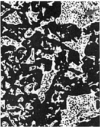
Fig. 2 Cross section of +40 mesh sponge iron obtained by reduction of ground magnetite. 125×
