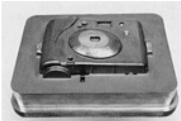
Fig. 9 An example of rapid tooling produced by LPM. Courtesy of J.A. Thomas, The Pennsylvania State University
