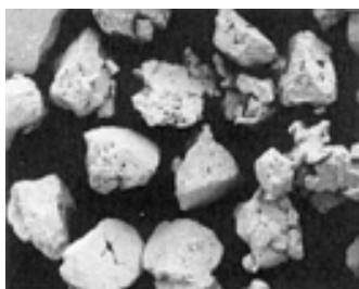
Fig. 29 Particles (+8 mesh) of copper powder hammer milled from oxide-reduced sinter cake. Courtesy of SCM Metal Products
