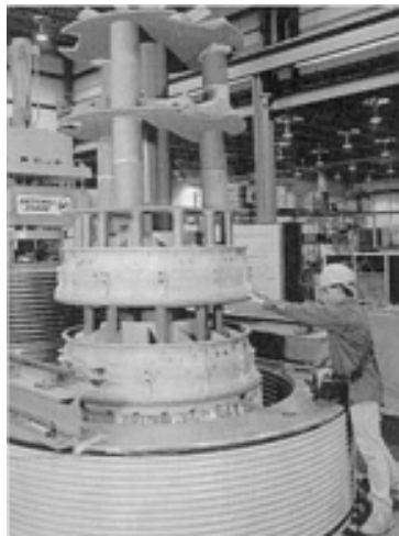
Fig. 2 Large HIP unit. 1.5 m (60 in.) diameter by 3.0 m (120 in.) work zone. Operating pressure: 100 MPa (15 ksi)
