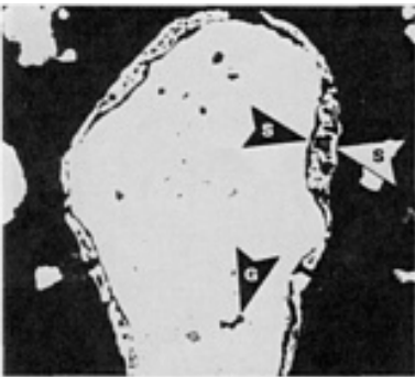
Fig. 153 Ancorsteel 1000 water-atomized, annealed iron. Solid particle with some gas porosity (arrow G) and some surface porosity (arrows S) caused the reduction of oxides picked up during atomization. As-polished. 645x
