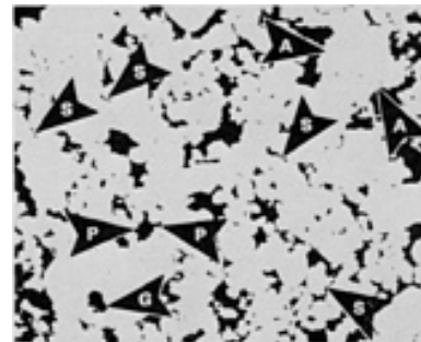
Fig. 51 Ancorsteel 1000 atomized iron powder ( 6.7 \text{ g/cm}^3 ), pressed at 410 to 480 MPa (30 to 35 tsi) and sintered 30 min at 1120 \text{ }^\circ\text{C} ( 2050 \text{ }^\circ\text{F} ) in dissociated ammonia. Arrows S indicate residual particle boundary segments. Dark regions (arrows P) are pores. Arrows A surround a solid atomized particle. Arrow G shows a pore inside a particle formed during atomization. As-polished. 120\times
