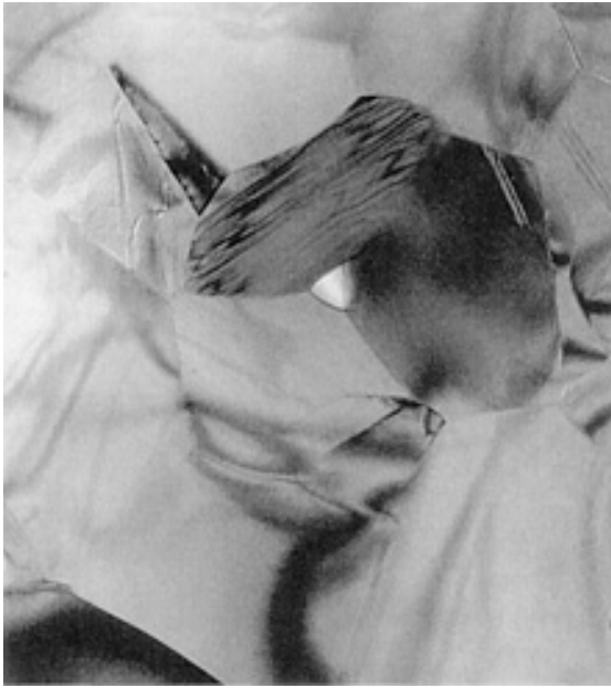
Fig. 3 Transmission electron micrograph of aluminum nitride sintered by PAS. Courtesy of T.A. Guiton, Dow Chemical Company. 69,000 \times
