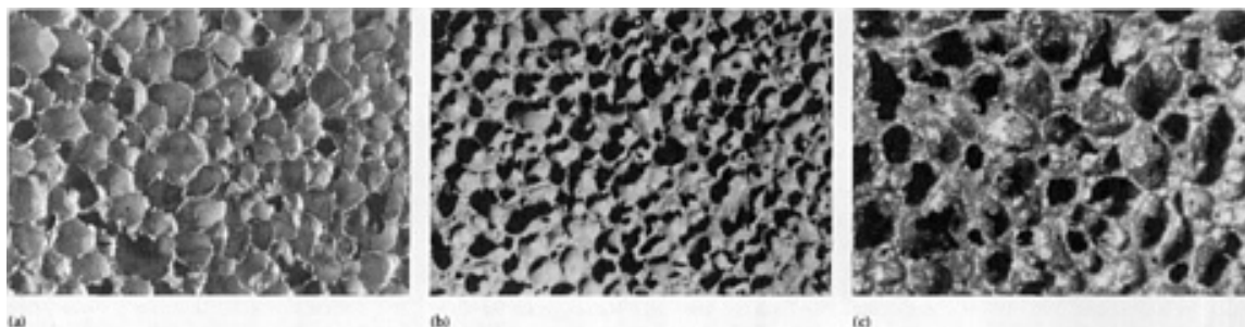
Fig. 1 Optical micrographs of (a) aluminum (4 to 1), zinc (6 to 1), and lead (4 to 1) foams
