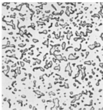
Fig. 12 Microstructure of silver-infiltrated 80W-20Ag billet. Angular microconstituents are silver. 500× Source: Ref 42
