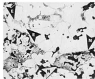
Fig. 95 Nickel steel (4% elemental carbonyl nickel admixed with atomized iron and 0.2% C, 6.7 \text{ g/cm}^3 ). See Fig. 86 for processing. Arrows E show a small colony of eutectoid, but most of the carbon is tied up in the nickel-rich regions (arrows N). Background is white ferrite grains. 2% nital. 330 \times
