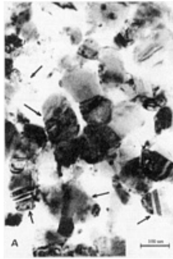
Fig. 14 Bright-field transmission electron microscopy image of 58 nm copper powder cold compacted at 750 MPa. Arrows indicate deformed particles presenting flat surfaces. Source: Ref 41
