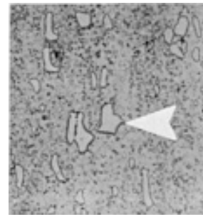
Fig. 114 Wrought T15 steel. Arrow shows large primary M 6 C carbide (compare with P/M tool steels in Fig. 115 and 116). Fine precipitate is vanadium carbide; matrix is martensite. 5% nital. 365x. (Ref 12)
