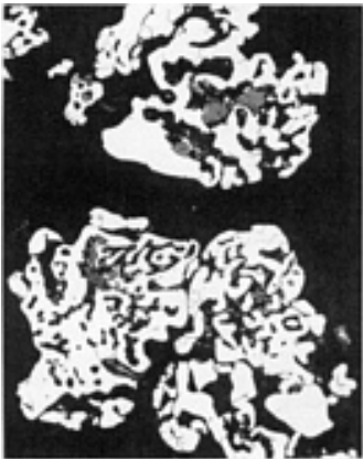
Fig. 3 Cross section of sponge iron particles. Etched with 2% nital. 180×
