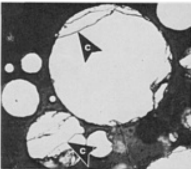
Fig. 159 Fe-31Si, water-atomized master-alloy powder (-100 mesh). Regular particle shape implies low green strength. Particles cracked (arrows C) during processing. As-polished. 645x
