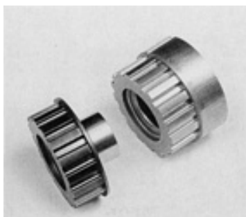
Fig. 1 Iron-carbon P/M drive gear. (a) Finished machined, hardened, ground part. The hub diameter is machined oversized (+0.254 mm, or +0.010 in.) to allow for final grinding. (b) P/M blank as-pressed
