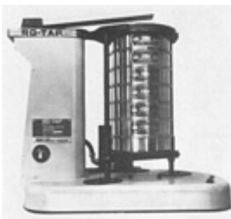
Fig. 16 Stacked sieves on a shaker with rotary and tapping action
