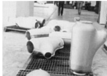
Fig. 23 Tees for underwater applications in the offshore industry hot isostatically pressed in 254 SMO grade. Weight: 155 kg/pc
