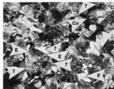
Fig. 90 Same as Fig. 88, but etched. The 2% Cu causes the nickel to dissolve, eliminating the nickel-rich regions. Arrows ? surround regions where the nickel probably was. These regions are darkened by the coring caused by copper dissolving there and contain carbide platelets. Another cored region is marked Co. Arrows E mark unresolved eutectoid, and arrow F indicates a white ferrite grain. 2% nital. 310\times
