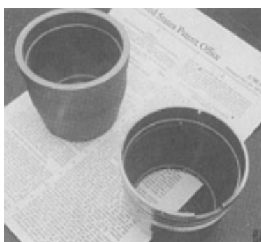
Fig. 5 Sidewinder missile component fabricated by the CHIP process. The left part is the near-net machining preform; the right part is the finished machined component. Courtesy of Dynamet Technology
