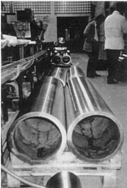
Fig. 7 Spray formed tubes of In625 alloy. Source: Osprey Metals, Ltd.
