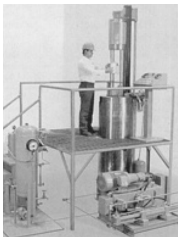
Fig. 3 Small CIP system with quick-opening top closure. Courtesy of EPS Inc.
