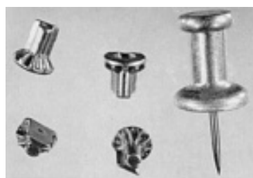
Fig. 10 Stainless steel gears for an electric toothbrush
