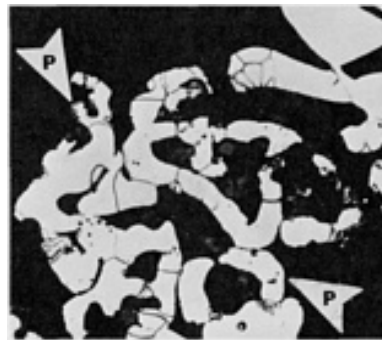
Fig. 151 MH-100 carbon-reduced sponge iron powder (-100 mesh). A few ferrite grain boundaries are shown, but no iron carbides. Arrows P surround a particle having extensive internal porosity. As-
