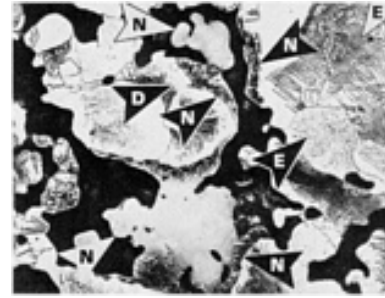
Fig. 94 Same as Fig. 93, but at higher magnification. Arrows N outline a nickel-rich region running through the structure along the pore surfaces, which probably forms a continuous three-dimensional network within the steel. Martensite needles are visible on the surface of the region. Arrows E show eutectoid; arrow D, white diffusion layer. 2% nital. 550 \times
