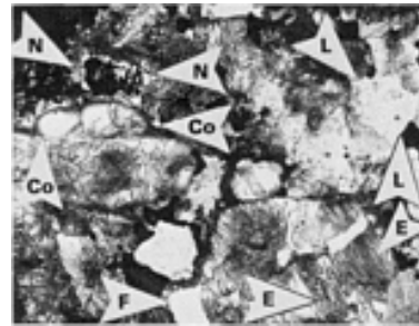
Fig. 89 Same as Fig. 87, but etched. Arrows N show nickel-rich region, inside which are martensite platelets. The effect of the 1% Cu is indicated by shading or coring of the ferrite (arrows Co). Arrows E show eutectoid; arrows L, an underetched region of eutectoid. Arrow F indicates a white ferrite grain. 2% nital. 310\times
