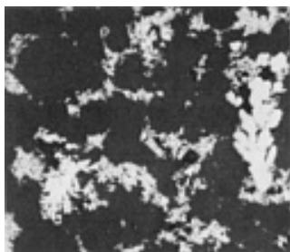
Fig. 4 Electrolytic copper powder, showing dendritic structure. 85×
