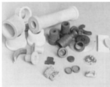
Fig. 21 Ceramic materials and net-shape articles produced by combustion synthesis
