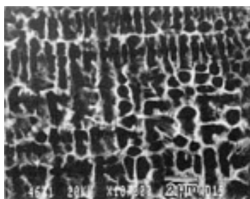
Fig. 13 A representative cell structure of carbides in a water-atomized high-speed steel powder cold sintered at 400 °C (SEM)
