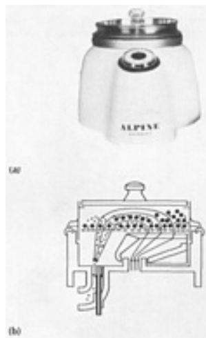
Fig. 2 Micromesh vacuum siever. (a) Apparatus. (b) Sectional view
