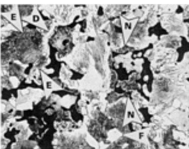
Fig. 92 Same as Fig. 91, but with 0.5% C. Arrows N outline nickel-rich regions. The fine structure within these regions is martensite and bainite. Arrows E outline a eutectoid region. Arrow F indicates a white ferrite grain. Arrow D shows a white diffusion layer between the eutectoid and the nickel-rich areas. 2% nital. 310 \times
