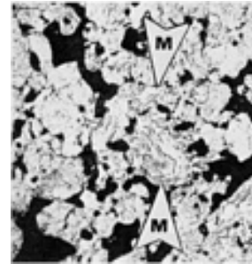
Fig. 113 Same type 410 stainless steel and pressing conditions as described in Fig. 112, but sintered 30 min at 1120 °C (2050 °F) and etched. Structure is all martensite (arrows M). Glyceregia. 545x
