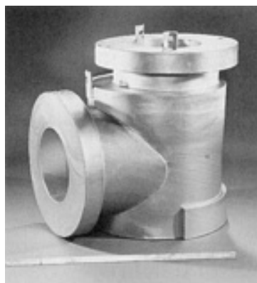
Fig. 24 Hot isostatically pressed valve body in austenitic stainless steel. Weight: 2 t
