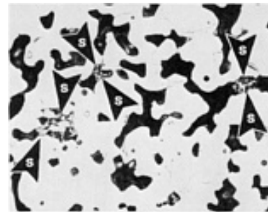
Fig. 85 Carbon-reduced sponge iron powder with 0.5% S blended as elemental fines. See Fig. 81 for processing ( 6.4 \text{ g/cm}^3 with 103 MPa, or 15 ksi, minimum yield strength). Arrows S show two-phase sulfide mixtures of MnS and FeS, which lie within the pores. 2% nital. 330\times
