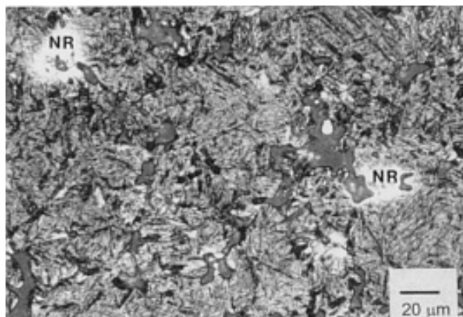
Fig. 16 Nickel-rich regions (NR) in a tempered martensitic structure of a quench-hardened and tempered P/M nickel steel (FN-0208)
