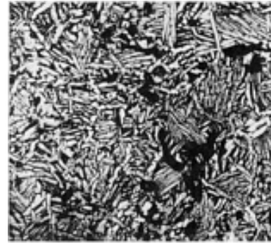
Fig. 124 Same as Fig. 123, but etched. Dark areas are residual rounded pores. Matrix is transformed \beta -titanium. 85 mL H 2 O, 5 mL HNO 3 , and 10 mL HF. 180×. (Ref 13)
