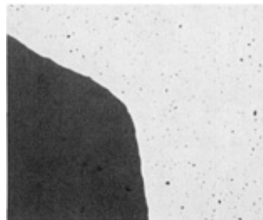
Fig. 131 Nickel steel (carbonyl Fe, 2% carbonyl Ni, and 0.3% C) injection molded and sintered (1120 °C, or 2050 °F) to 97% density. Structure shows fine isolated
