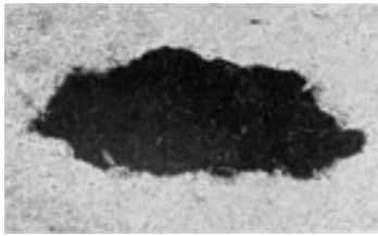
Fig. 6 Iron powder contamination of water-atomized low-alloy steel powder. Source: Ref 21
