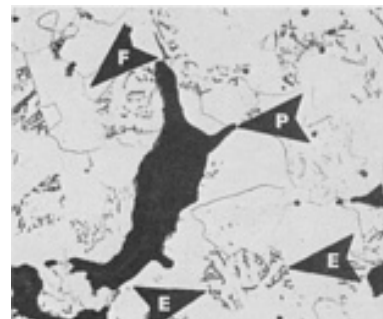
Fig. 76 Prealloyed, low-alloy steel (Fe-1.85Ni-0.60Mo-0.2C, 6.7 g/cm 3 ), processed as per Fig. 73. Matrix is white ferrite (arrow F). Eutectoid is found in colonies (arrows E).
