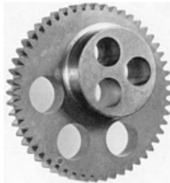
Fig. 4 Eccentric gear for a washing machine made of iron alloy powder containing 2% copper and 0.5% graphite. Center hole inside diameter: approximately 19 mm (0.76 in.); eccentric outside diameter: approximately 57 mm (2.28 in.); total thickness: approximately 28.50 mm (1.14 in.); eccentric thickness: approximately 15.90 mm (0.63 in.); pitch diameter: approximately 115 mm (4.59 in.)
