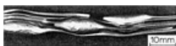
Fig. 13 Attempt to coreduce cast cobalt alloy rods in low-carbon steel matrix. See Fig. 14.
