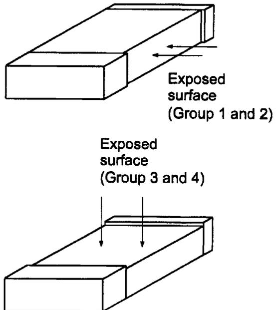
Fig. 3 Principle of exposure of test samples.
