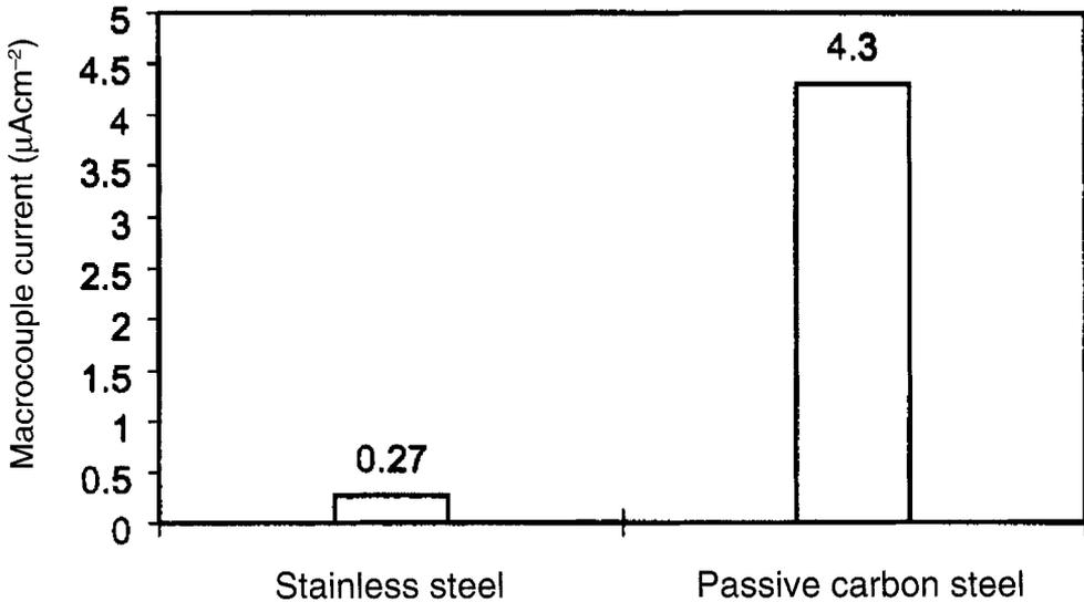
Fig. 5 Macrocouple current for stainless steel and passive carbon steel.
