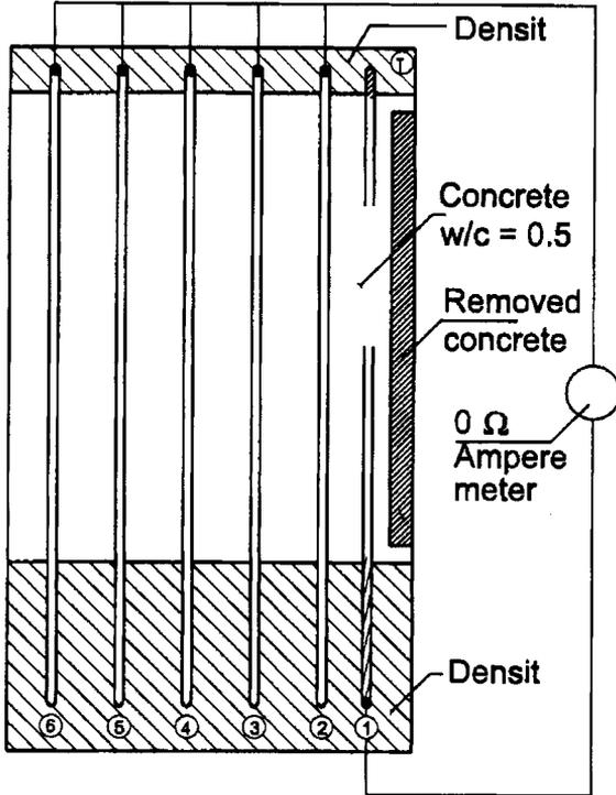
Fig. 2 Sketch of test samples.
