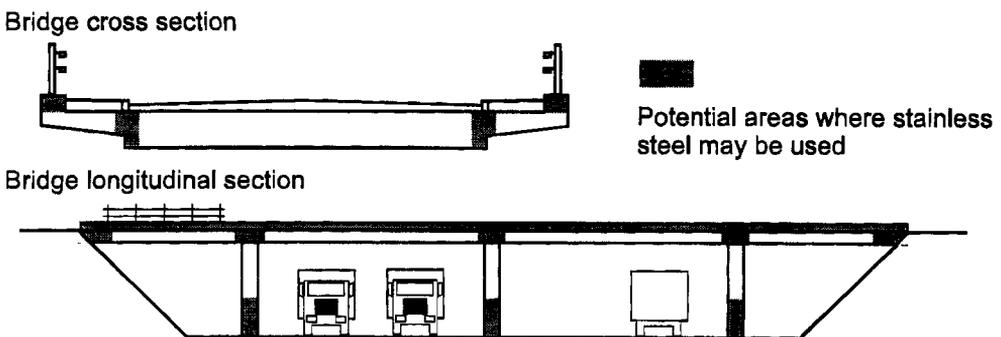
*Fig. 1 Potential areas where stainless steel may be used intelligently for repair and in new structures as well.*
