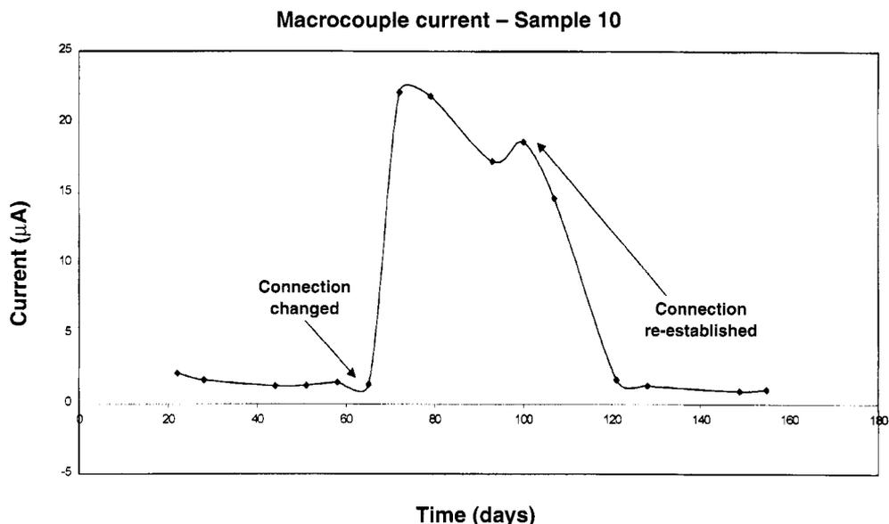
*Fig. 6 Influence of cathode material on the macrocouple current (see p.127).*
