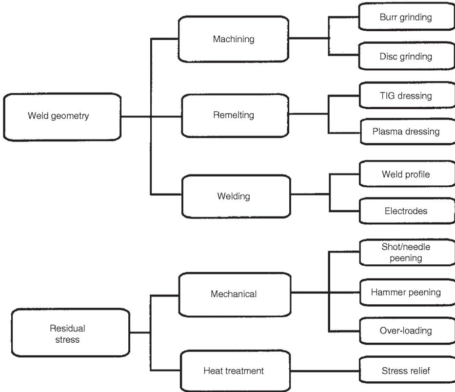
**Fig. 24** Range of postweld fatigue life improvement techniques. TIG, tungsten inert gas. Source: Ref 16
