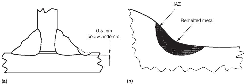
**Fig. 25** Typical profiles for (a) burr grinding and (b) gas tungsten arc weld dressing of weld toe. HAZ, heat-affected zone. Source: Ref 16
