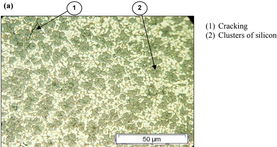
Fig. 1 (a) 431 alloy (Al 29.8Si 1.3Cu 1.4Mg 0.3Fe 0.3Ni 0.3Zr) flake optical micrograph etched, air side longitudinal cross-section, (b) 461 ribbon (Al 21Si 3.9Cu 1.2Mg 2.4Fe 1.4Ni 0.4Zr) optical micrograph longitudinal section.
