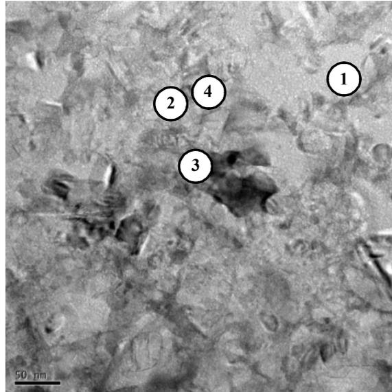
Fig. 3 TEM micrograph of 461 (Al 21Si 3.9Cu 1.2Mg 2.4Fe 1.4Ni 0.4Zr) ribbon unetched. Points 1,2,3,4 and 2 were analysed by EDX (see Fig. 4)
