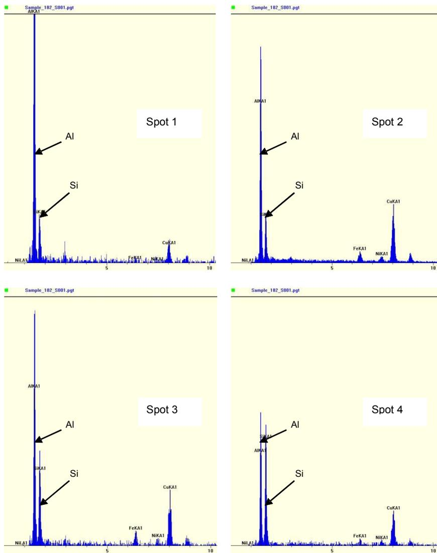
Fig. 4 EDX spectra for points 1, 2, 3 and 4 in Fig. 3, showing relatively high Al in points 1 and 2 and relatively higher Si for points 3 and 4.
