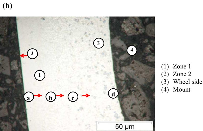
Fig. 2 FEGSEM backscattered micrograph of 461 ribbon (Al 21Si 3.9Cu 1.2Mg 2.4Fe 1.4Ni 0.4Zr) unetched.
