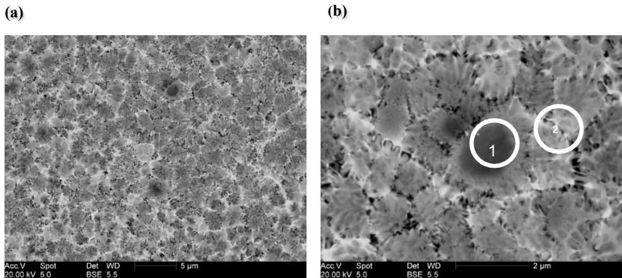
Fig. 5 FEGSEM backscattered electron micrographs of 461 (Al 21Si 3.9Cu 1.2Mg 2.4Fe 1.4Ni 0.4Zr) ribbon.
