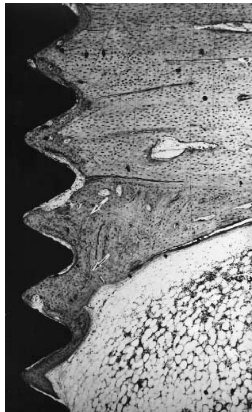
Fig.4 In biomaterials science, osteoconduction means growth of bone on the surface of a foreign material, as seen in the lower part of this titanium screw implant (arrows). Distance between thread peaks, 600 \mu\text{m}
