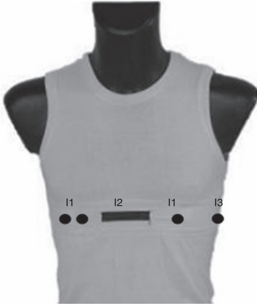
12.3 The first PROeTEX inner garment with: I1 – textile electrode for measuring heart rate; I2 – piezoresistive sensor for measuring breathing rate; I3 – thermocouple for measuring body temperature.
