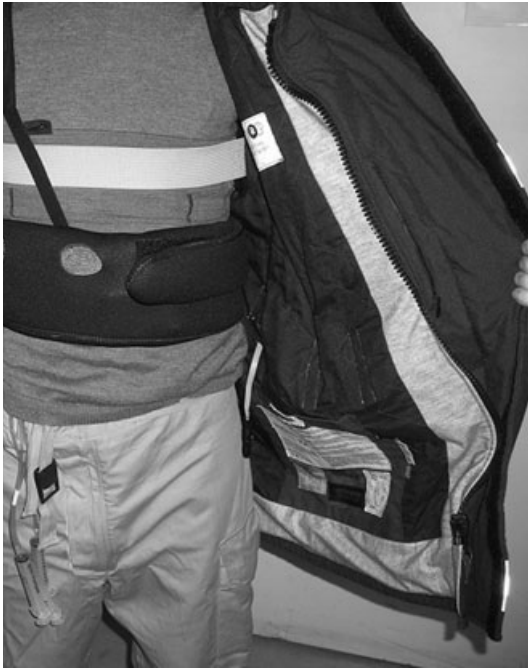
12.5 Belt with piezoelectric sensor and vital signs board (VSB), wirelessly connected to the Personal Electronic Box (PEB).
