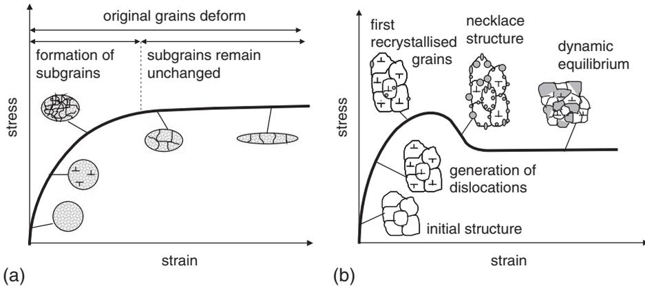
**Figure 5.8.** Evolution of the microstructure during (a) hot deformation of a material showing recovery and (b) dynamic recrystallization or discontinuous dynamic recrystallization.
