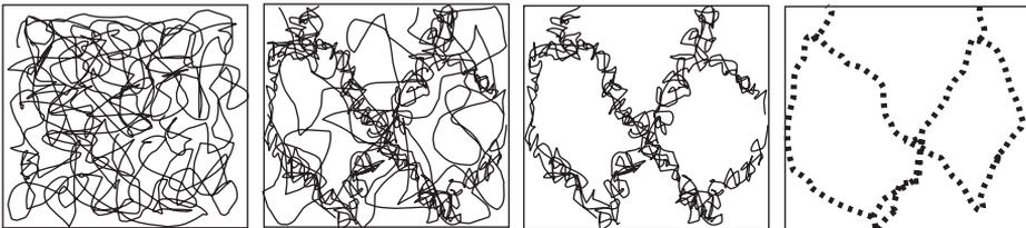
**Figure 5.4.** Schematics showing dislocation structure changes during recovery – random dislocation tangles through cell structures to subgrains.
