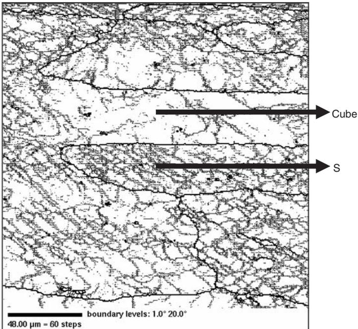
**Figure 5.5.** Difference in substructure between Cube  $\{001\}\langle 100\rangle$  and S  $\{231\}\langle 346\rangle$  in aluminum – EBSD measurement on hot worked AA 1050 (Samajdar *et al.* [2001]).
