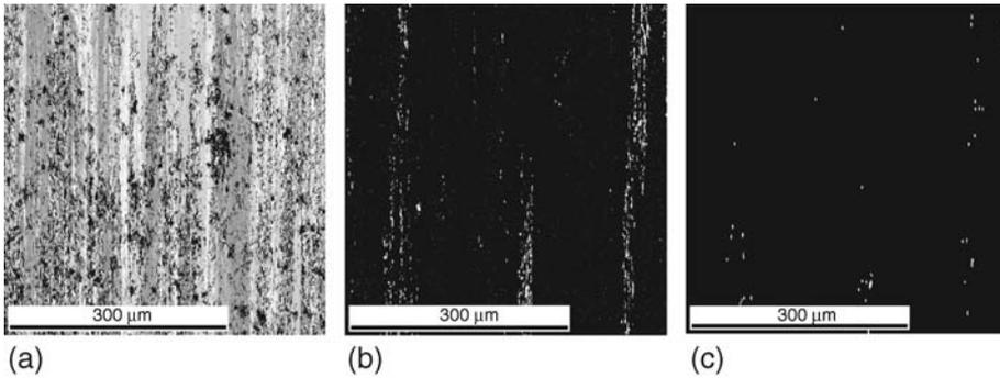
**Figure 5.6.** EBSD images of (a) hot deformed aluminium, (b) deformed Cube grain in (a), and (c) recrystallized Cube grain in (a). Distinction between (b) and (c) was established by considering grain orientation spread and grain size. A comparison of (b) and (c) indicates that the recrystallized Cube originate from deformed Cube. Courtesy Ravindra (IIT Bombay) – Research in Progress.
