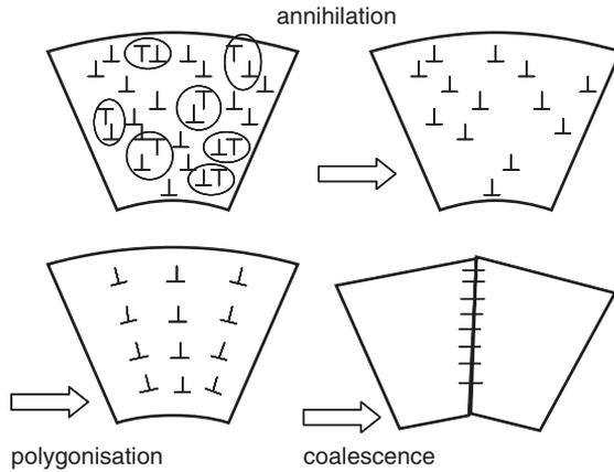
**Figure 5.2.** Schematic of successive dislocation annihilation mechanisms; cross-section of a bent crystal containing both free (edge) dislocations and dislocations, which accommodate the orientation gradient. During annealing, some dislocations anneal out by climb of opposite sign segments (encircled pairs) then the remainder rearrange into subgrain boundaries.
