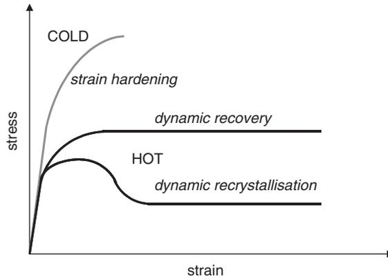
**Figure 5.7.** Typical flow curves during cold and hot deformation.
