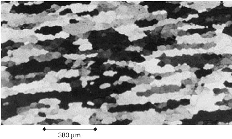
**Figure 5.9.** Polarized light optical image of hot deformed aluminium showing serrated grain boundaries (Samajdar *et al.* [2001]).
