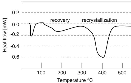
**Figure 5.3.** DSC plots at 20 K/min of ultrahigh purity Fe cold rolled 80% (Scholz *et al.* [1999]). Negative heat flows correspond to exothermic reactions, which are estimated at  $\approx 4$  J/mol for the recovery region (100–300°C) and 15 J/mol for recrystallization (320–450°C).
