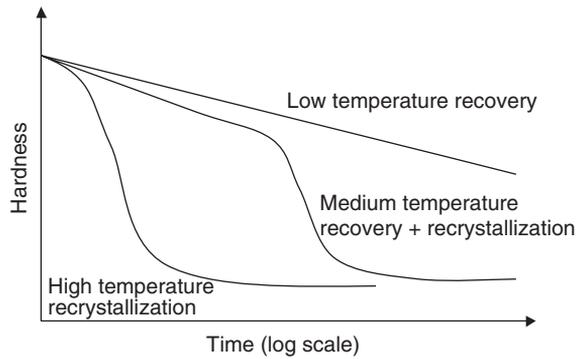
**Figure 5.1.** Schematic softening kinetics at three temperatures for different combinations of recovery and recrystallization.
