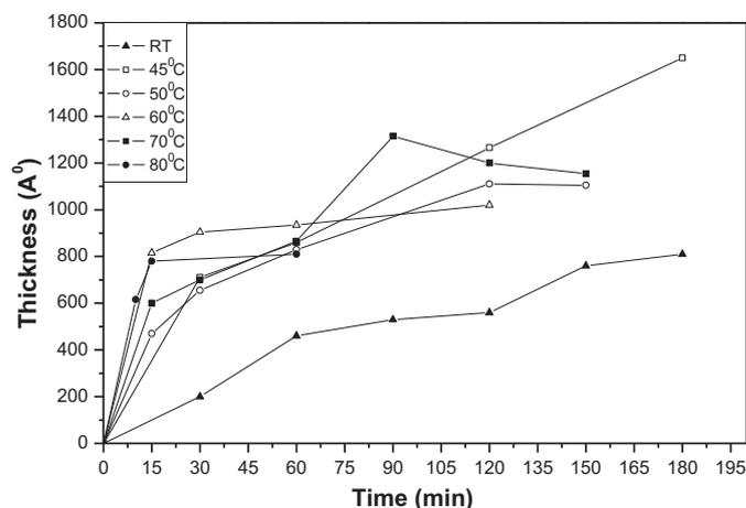
Fig. 1. Thickness variation as a function of time at different bath temperatures. Bath composition:  $[\text{ZnSO}_4] = 0.05$  M,  $[\text{TA}] = 0.02$  M,  $[\text{NH}_3] = 9.8$  M.
