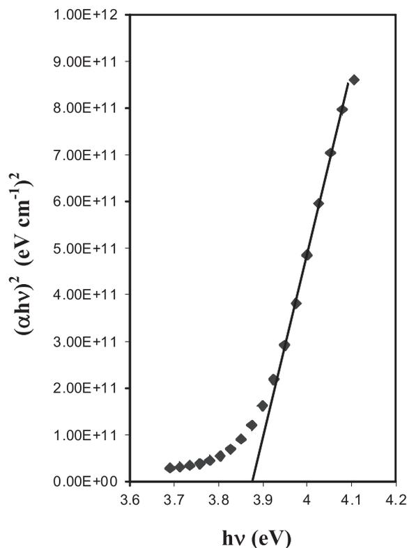
Fig. 10. (αhv)<sup>2</sup> Versus hv plot for a typical CBD ZnS film deposited under optimized conditions: [ZnSO<sub>4</sub>] = 0.05 M, [TA] = 0.04 M, [NH<sub>3</sub>] = 9.8 M and t<sub>b</sub> = 60 °C.
