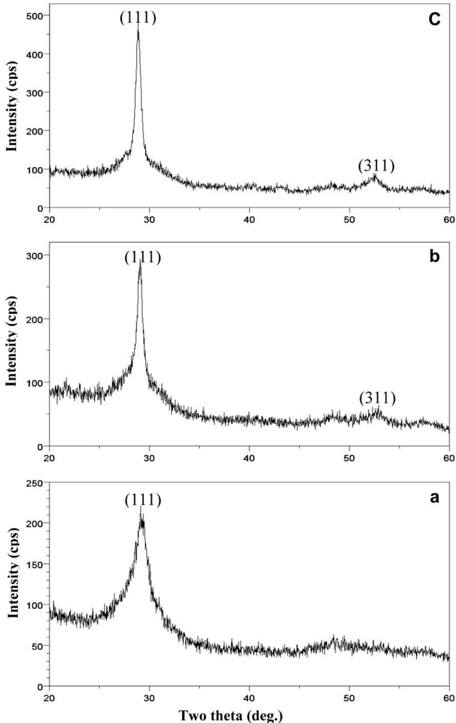
Fig. 5. GIXRD pattern of CBD ZnS films deposited from chemical baths with different thioacetamide concentrations keeping  $[ZnSO_4] = 0.05$  M,  $[NH_3] = 9.8$  M and  $t_b = 60$  °C. (a)  $[TA] = 0.02$  M, (b)  $[TA] = 0.04$  M, (c)  $[TA] = 0.06$  M.
