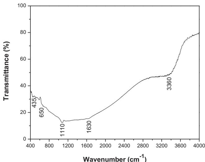
Fig. 8. FTIR spectrum of a typical ZnS film deposited under optimized conditions: [ZnSO<sub>4</sub>] = 0.05 M, [TA] = 0.04 M, [NH<sub>3</sub>] = 9.8 M and t<sub>b</sub> = 60 °C.
