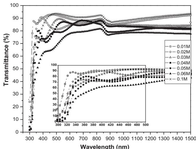
Fig. 9. Transmission spectra of CBD ZnS films deposited with different thioacetamide concentrations. Inset: Expanded view of the fundamental absorption region.
