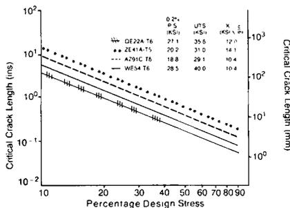
Figure 5. Critical crack lengths as a function of percentage design stress for various magnesium alloys.
