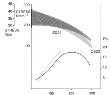
Figure 1. Effect of temperature on tensile properties of EQ21 vs. QE22.
