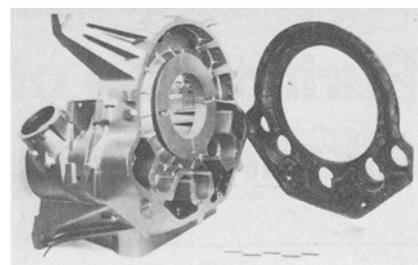
Figure 6. This casting, produced in ZE41, weighs 620 lbs. and is the main gearbox for the Westland WG34 helicopter.
