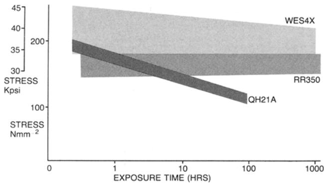
Figure 3. Effect of exposure time on tensile properties of 482°F (250°C) for WE54X compared with QH21A and Al casting alloy RR350.
