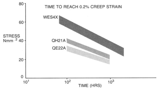
Figure 4. Stress/strain relationship for WE54 vs. QH21A and QE22A at 482°F (250°C).
