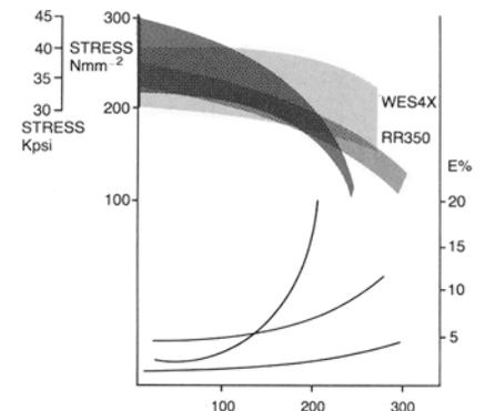
Figure 2. Effect of temperature on tensile properties of WE54 vs. the high temperature Al alloys RR350 and A356.
