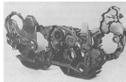
Figure 7. Shown is a sectioned gear casting, revealing cored passageways.
