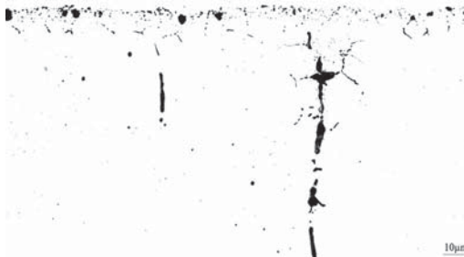
Figure 43 Extreme intergranular surface oxidation, as-polished surface, 14NiCr18.
