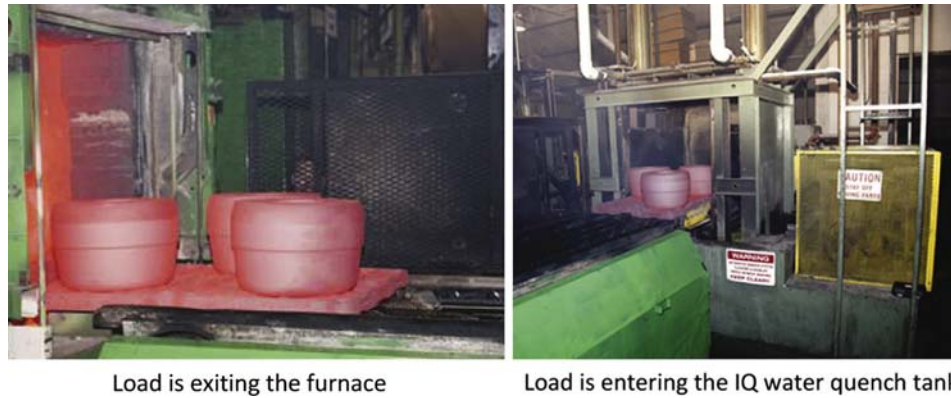
Figure 5 Production IQ system installed at Akron Steel Treating Co.
