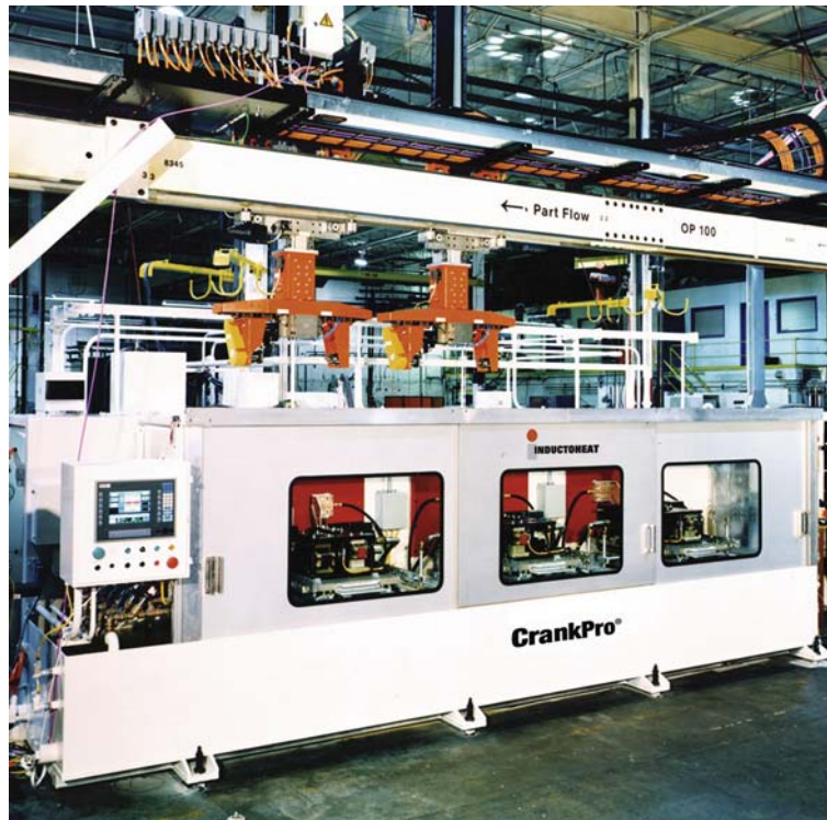
Figure 46 CrankPro machine implements Inductoheat's patented nonrotational crankshaft hardening and tempering technology (SHarP-C). Courtesy of Inductoheat, Inc.
