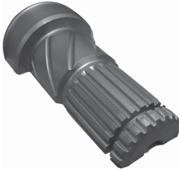
Figure 39 Representative part having various geometrical discontinuities. Reproduced from Rudnev, V. Computer Modeling Helps Prevent Failures of Heat Treated Components. Adv. Mater. Process. October, 2011 , 28–33.
