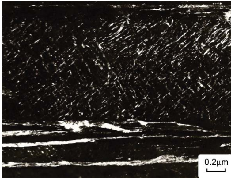
Figure 6 Transition carbides (the fine bright features) within a crystal of lath martensite and interlath retained austenite (the elongated bright features) in 4130 steel tempered at 150 °C. Dark-field transmission electron micrograph taken with diffracted beams from transition carbides and retained austenite. Courtesy of Mauro Losz.
