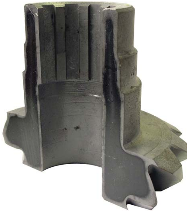
Figure 63 Spiral bevel pinion was induction hardened using TSH Technology. Courtesy of ERS Engineering Corp.
