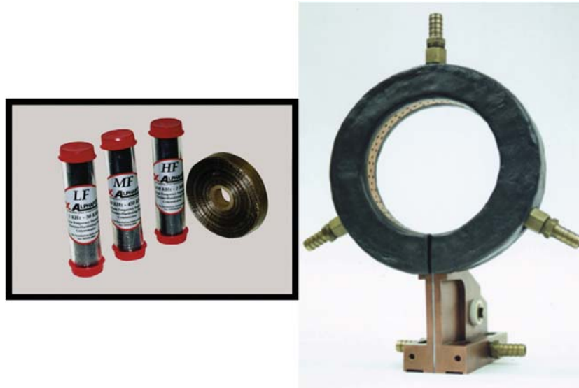
Figure 33 Some flux concentrator materials are supplied in a softened condition and can easily be formed into a shape sufficiently machined, if desired, to exact tolerances. Reproduced from Rudnev, V. An Objective Assessment of Magnetic Flux Concentrators. ASM Int., Materials Park, Ohio. Heat Treat. Prog. Nov./Dec., 2004 , 19–23.
