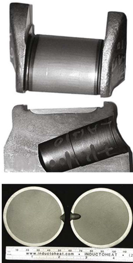
Figure 48 Nonrotational hardening process provides crankshaft pins and mains with superior microstructural properties. Reproduced from Doyon, G.; Brown, D.; Rudnev, V.; Desmier, G.; Elinski, J. Taking the Crank out of Crankshaft Hardening. Ind. Heat. December, 2008, 41–44.
