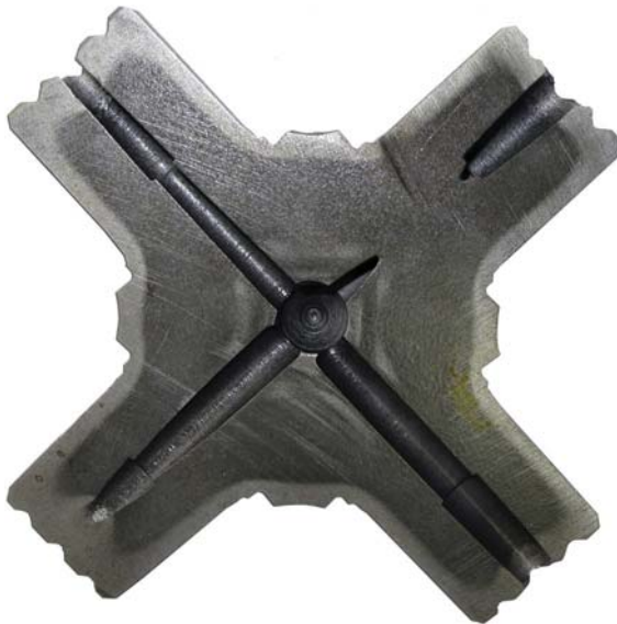
Figure 64 Automotive journal cross was induction hardened using TSH Technology. Courtesy of ERS Engineering Corp.
