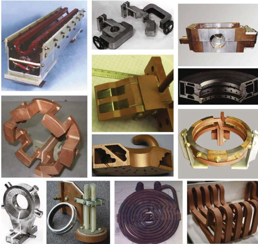
Figure 3 Specifics of the inductor design is typically application-oriented. Courtesy of Inductoheat Inc.
