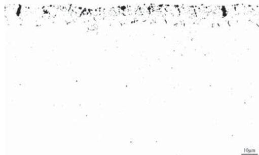
Figure 40 Intergranular surface oxidation, 15CrNi6, unetched microstructure.
