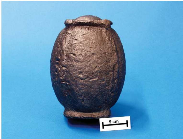
Figure 9 Dead-weight body after a few hundreds of passes through a heat treatment furnace. Original geometry: square billet (photo by Ulrich Reiß, IWT Bremen).
