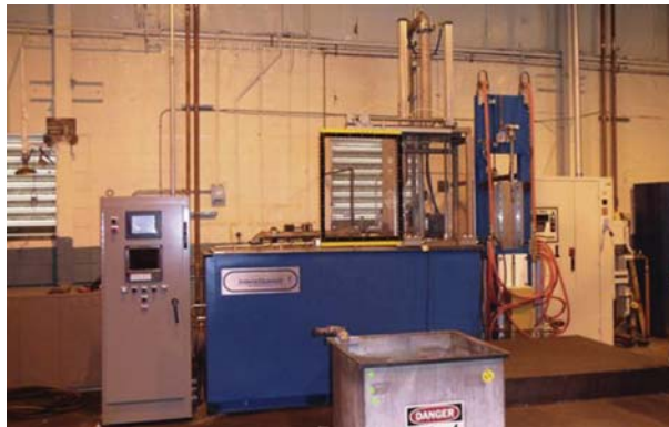
Figure 16 High-velocity IQ system for processing shafts of up to 50 mm diameter and 910 mm length installed at Euclid Heat Treating Co.
