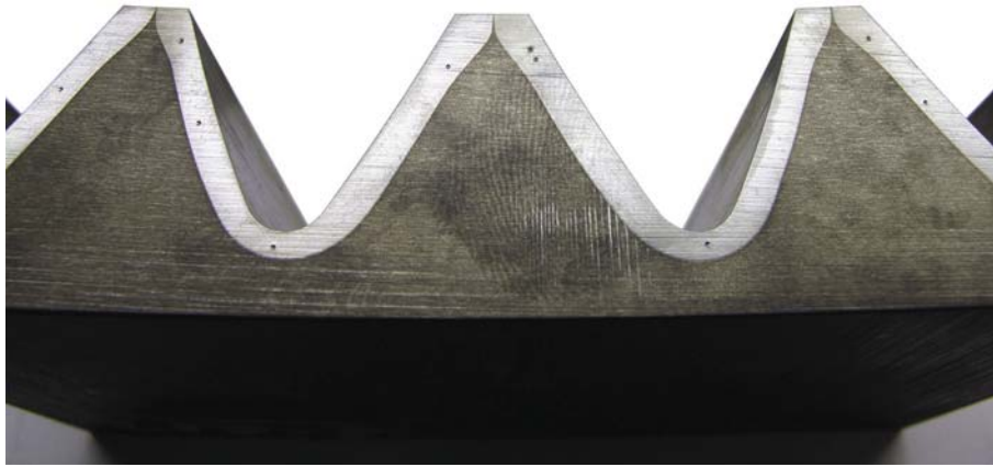
Figure 55 Gear-hardened pattern using gap-by-gap hardening. Courtesy of Inductoheat Inc.
