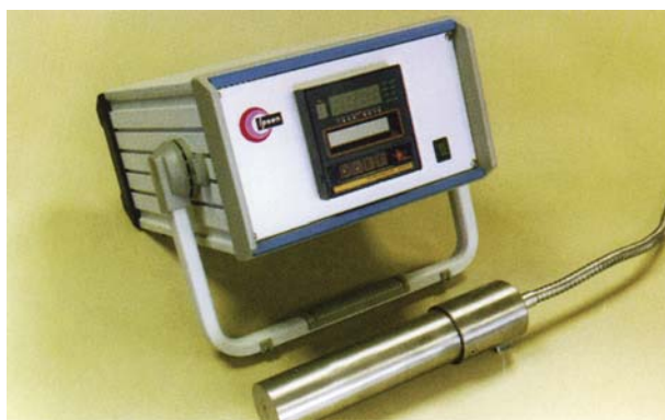
Figure 34 The data-logger with the Ipsen–Liscic sensor. By courtesy of Ipsen, GmbH, Kleve.
