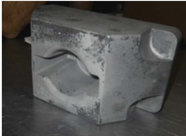
Figure 10 S5 punch intensively quenched by use IQ-2 process.
