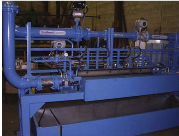
Figure 17 High-velocity IQ system for processing torsion bars.
