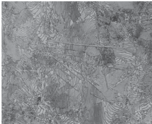
Figure 17 Microstructure of as-rolled Fe – 1.31% C – 0.35% Mn – 0.25% Si high-carbon water hardenable tool steel. Note the Widmanstätten intragranular cementite that precipitated as proeutectoid cementite before the eutectoid reaction. Originals at 1000 \times . 4% Picral etch. Courtesy of George Vander Voort.
