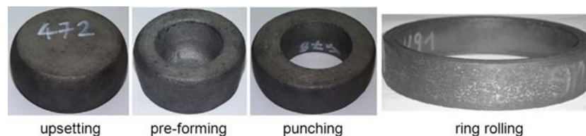
Figure 22 Process steps during hot forming (photo by Ulrich Reiß, IWT Bremen).
