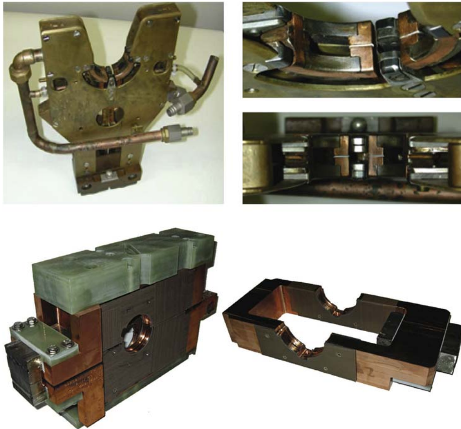
Figure 49 A side-by-side comparison of rigidity and complexity of U-shaped inductor (top) versus SHarP-C inductor (bottom). Reproduced from Rudnev, V.; Doyon, G.; Brown, D. Innovative Induction Heating Technologies. Pittsburgh. In Proc. of Materials Science & Technology Conf. (MS&T-08) ; 5–9 Oct., 2008.
