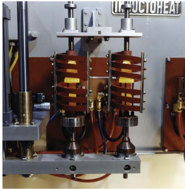
Figure 69 Simultaneous induction hardening of mining tool bits and brazing the working tips. Courtesy of Inductoheat Inc.
