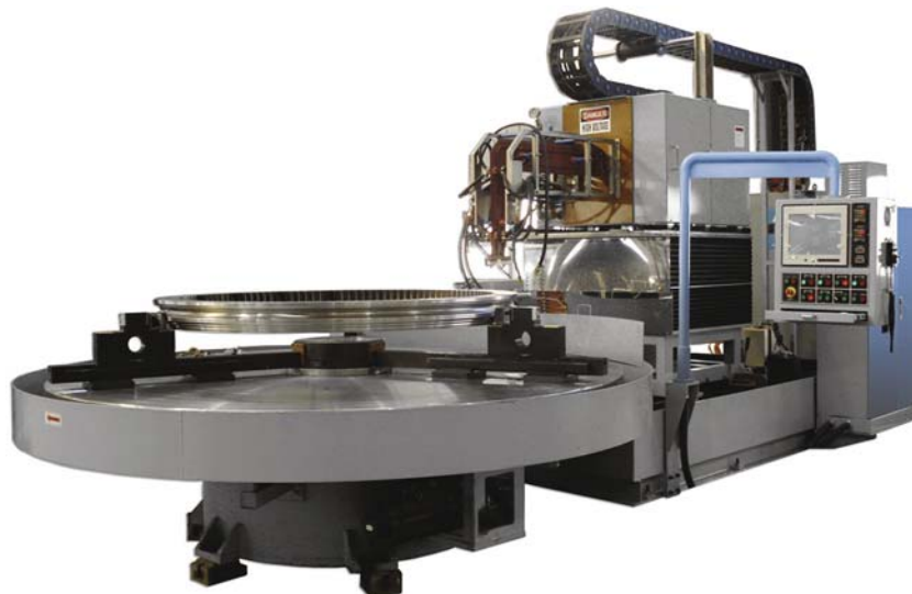
Figure 57 Induction gear-hardening machine for a large-diameter ring for a wind-turbine generator with teeth located on the inside diameter of the ring. The bearing ring OD can be as large as 3.5 m, the required case depth is 2.5–3.5 mm, the z-axis scan height (tooth width) is 350 mm, and the maximum weight exceeds 5 tons. Courtesy of Inductoheat-HWG, Germany.
