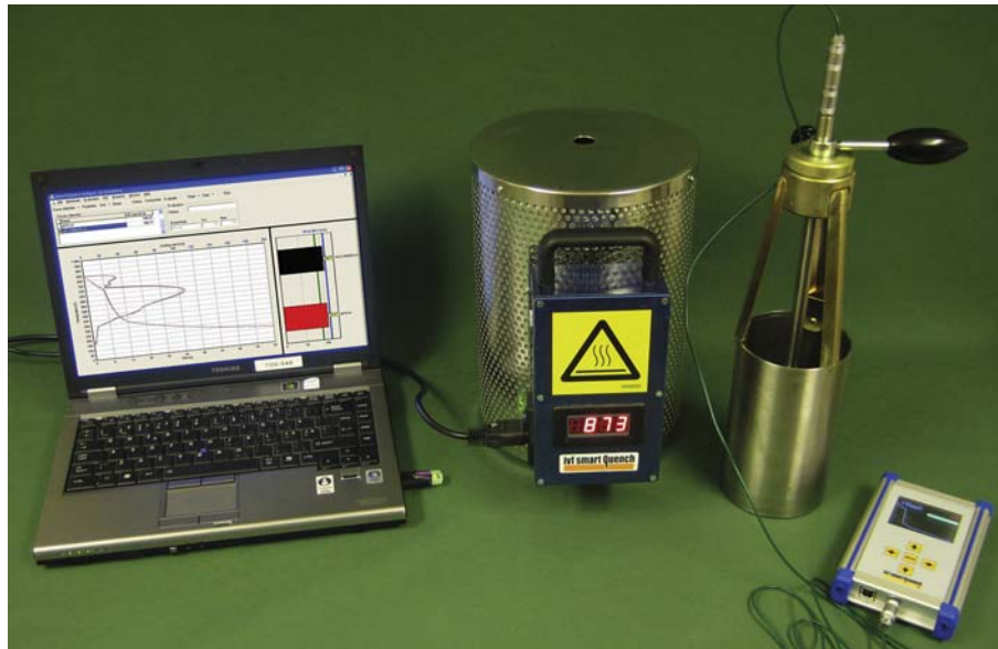
Figure 13 Equipment for standardized testing of quenchants (ivf SmartQuench). Reproduced from ivf SmartQuench, Users' Manual., Swerea IVF AB, 2009.
