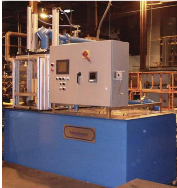
Figure 15 High-velocity IQ system for processing parts of up to 200 mm diameter and 500 mm length installed at Euclid Heat Treating Co.
