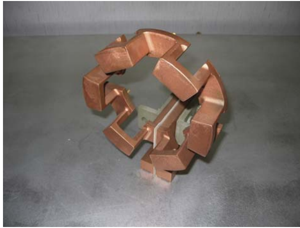
Figure 19 A single-shot inductor for hardening complex geometry component. Courtesy of Inductoheat Inc.
