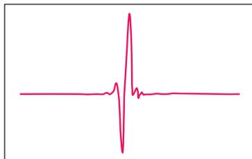
This means that as the interferogram is measured, all frequencies are being measured **simultaneously**. Thus, the use of the interferometer results in extremely fast measurements.
