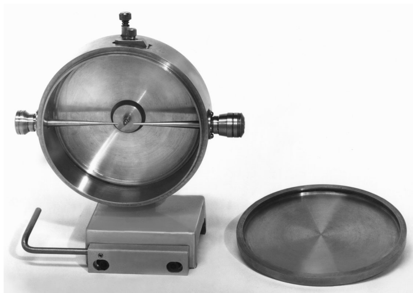
Figure 1 Hull/Debye-Scherrer camera, with cover plate removed. (Courtesy of Philips Electronic Instruments, Inc.)
